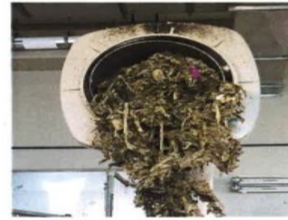
Photo of clogged wastewater equipment taken on March 17, 2020 from a sewage pumping station in London, Ontario. Photo credit Barry Orr and CWWA.
